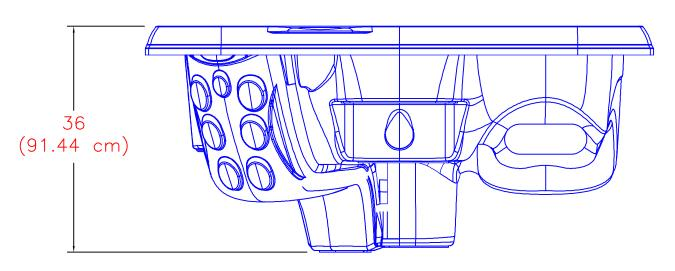
NOTE: Dimensional tolerances are as follows due to variations in manufacturing: Length / Width / Height(s): +/- 3/8" Height Variance (side to side): +/-1/4"
