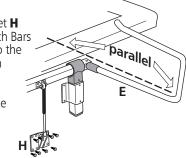
8. Affix each Black Plastic Bumper I to the spa cabinet by peeling off the adhesive strip and applying to the spa cabinet directly under the corner of the Catch Bar E, as shown. NOTE: The skirt must be clean and dry before applying the bumpers. (On oily surfaces, a screw or small nail may be required to hold the bumpers in place.)
