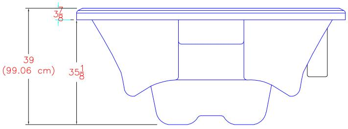
NOTE: Dimensional tolerances are as follows due to variations in manufacturing: Length / Width / Height(s): +/- 3/8" Height Variance (side to side): +/-1/4"
